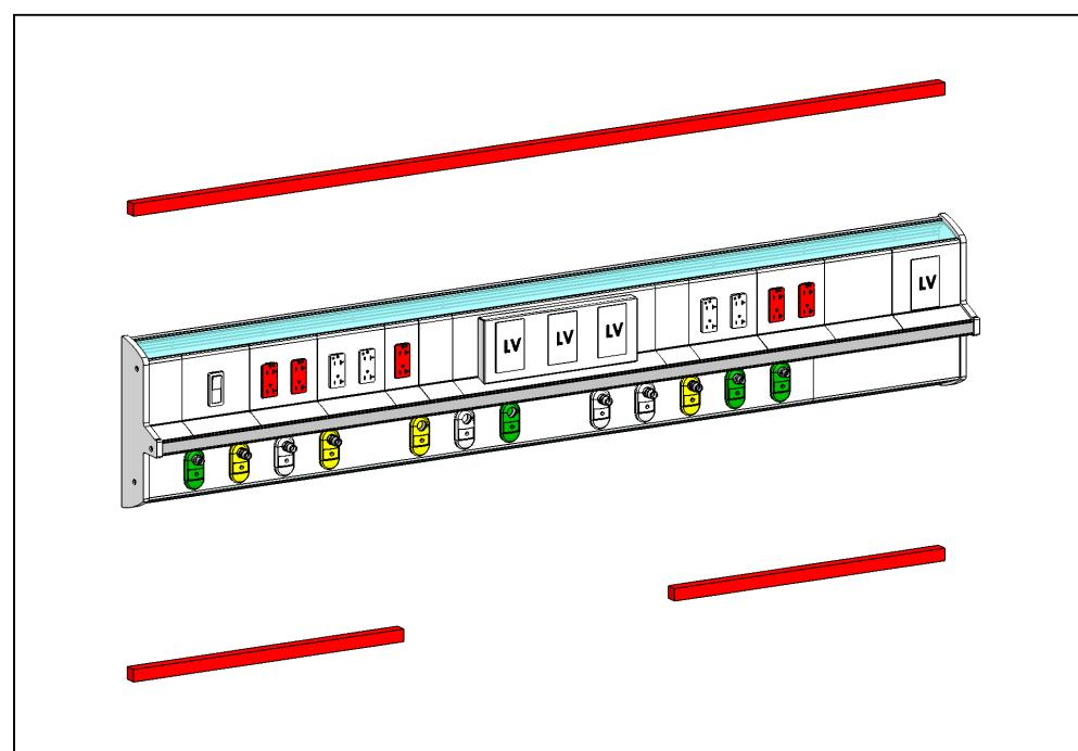
STANDARD 6 FOOT MEDICAL GAS RAIL HEADWALL ISOMETRIC VIEW
